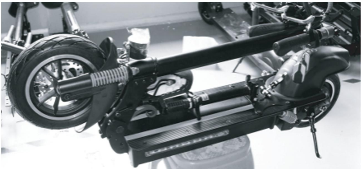
③ When you hear the sound, the folder is locked and the vertical pole is folded.
