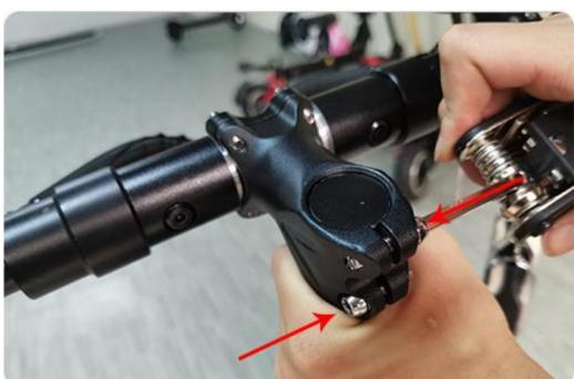
3. Adjust the angle and fasten itScrews,
