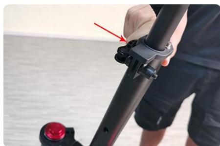
3. Press the lever lock switch to lock the lever
