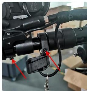
4. Check whether the brake handle, headlight switch, dual drive switch, and instrument are fixed.and fix the unfixed screw
