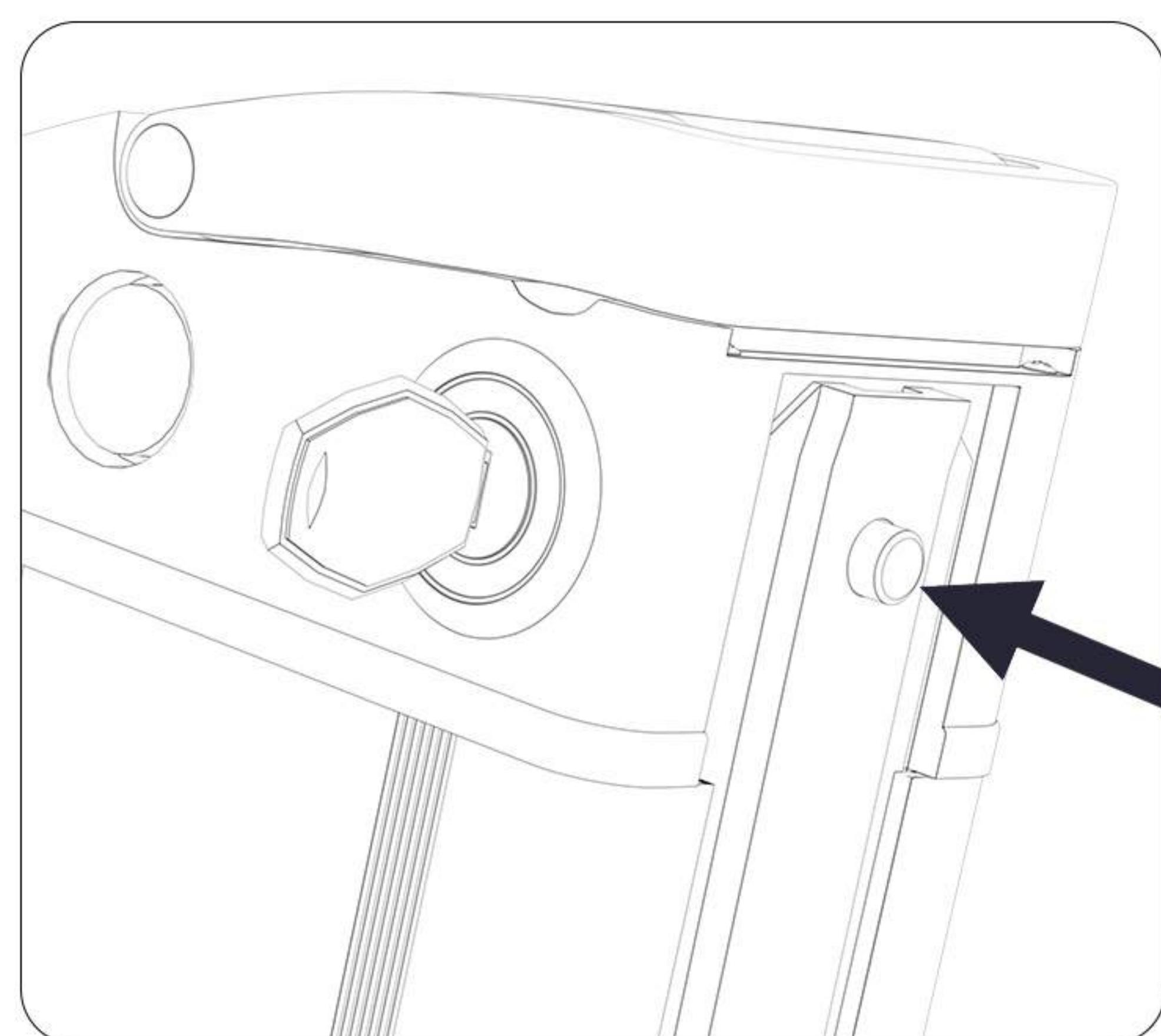
Position 1: In this position, the battery starts supplying power, and the key cannot be removed.
