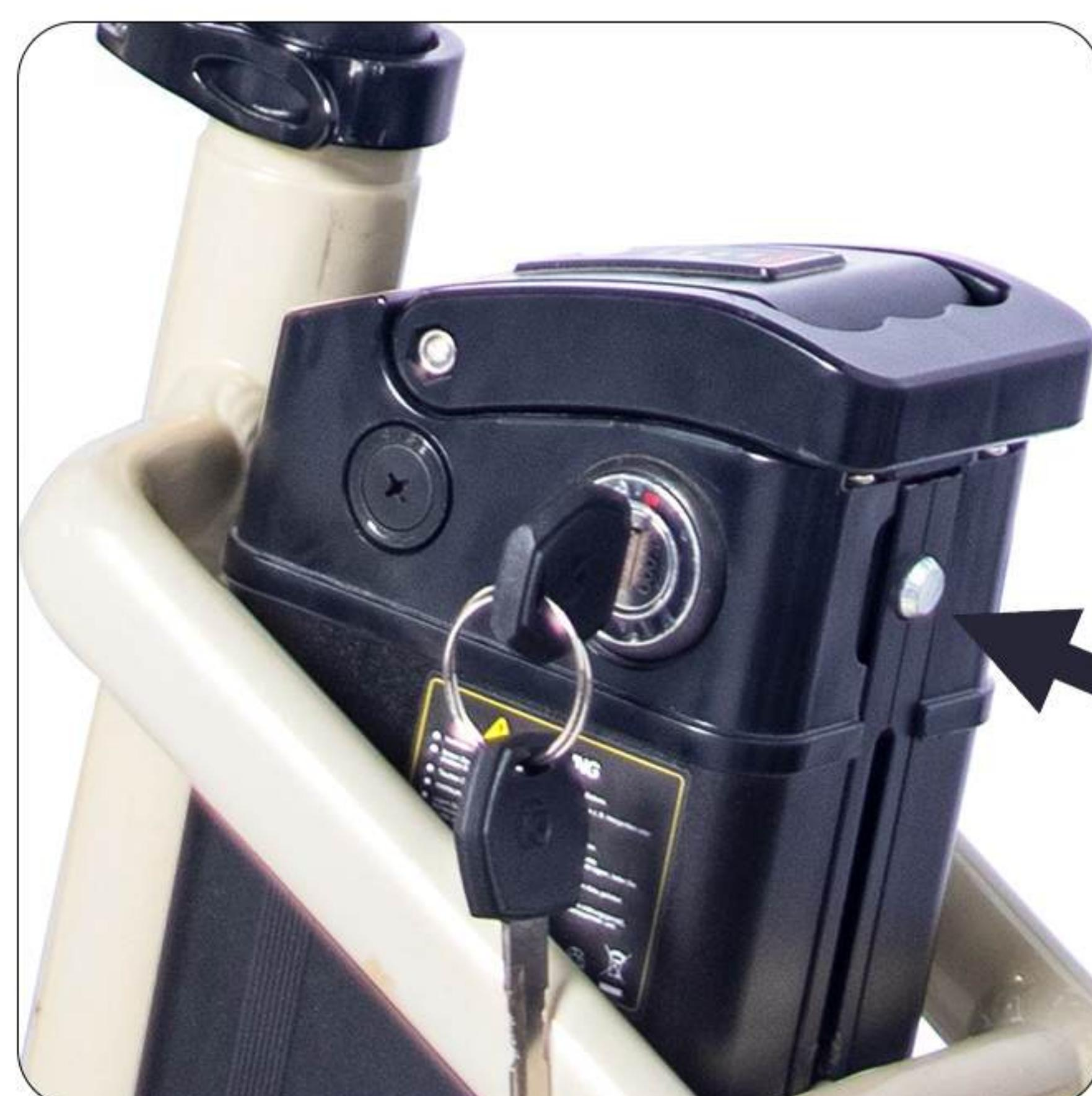
2. Turn the key to extend the rear latch and lock the battery.
