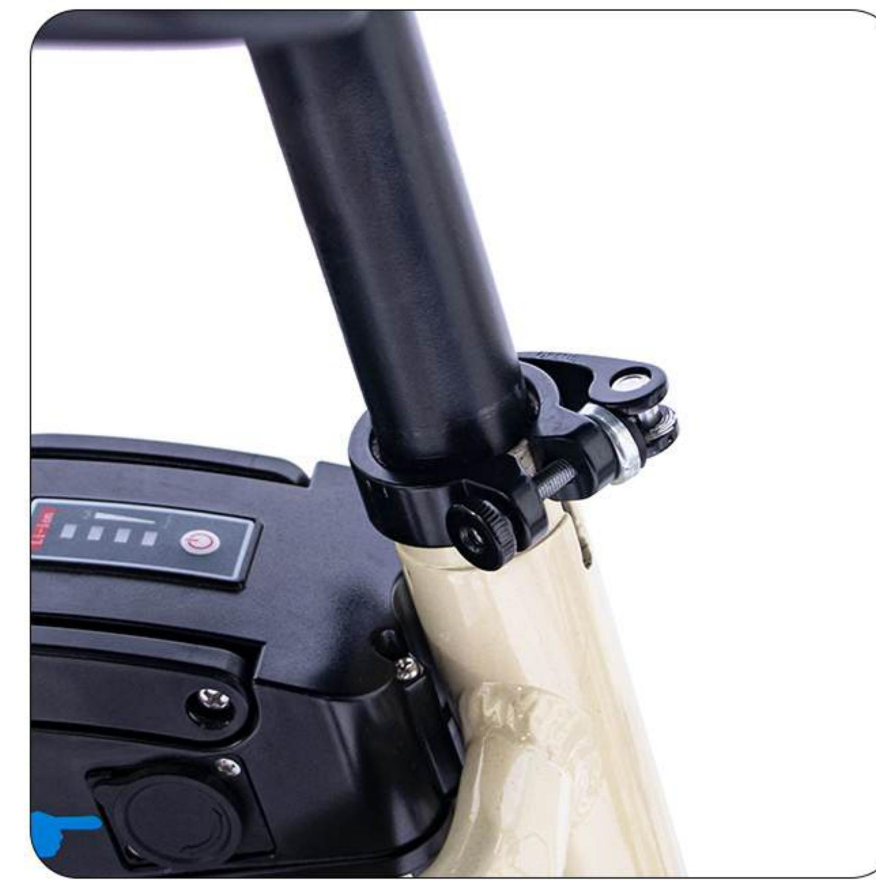
12. Loosen the seat buckle, install the seat, adjust the height, and then tighten the seat buckle.
