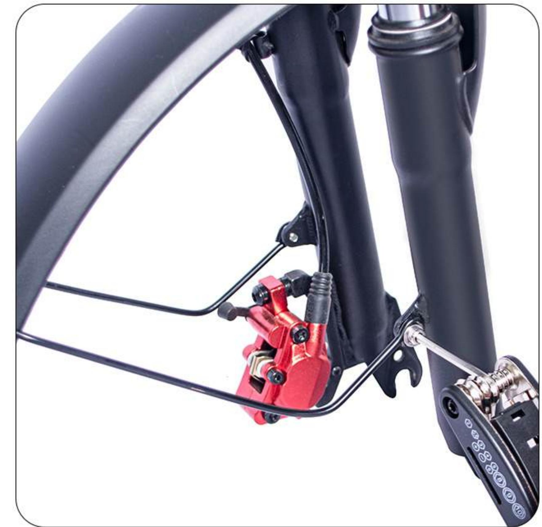
6. Install the two screws for the fender bracket.
