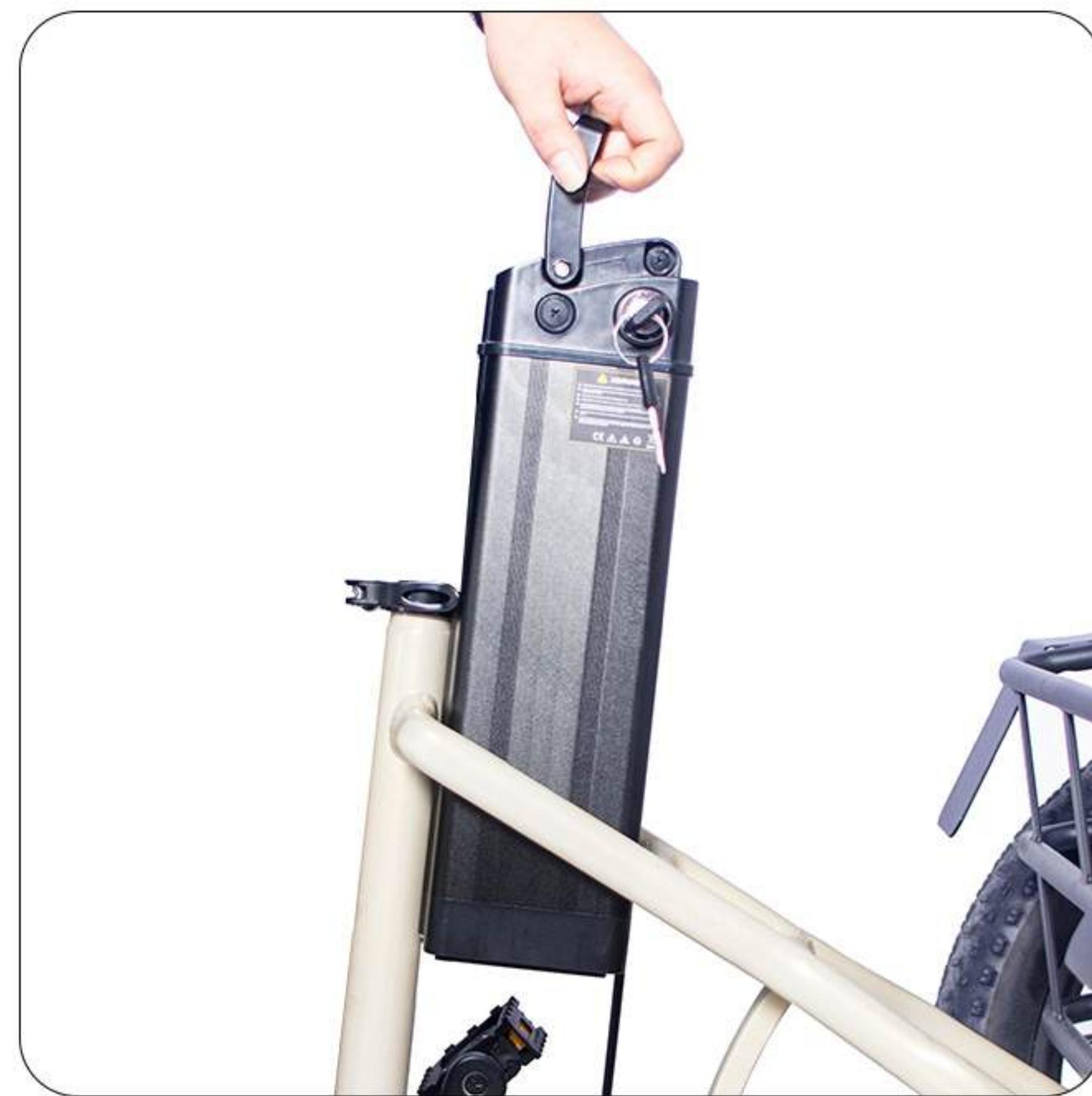
3. Pull upwards to remove the battery.
