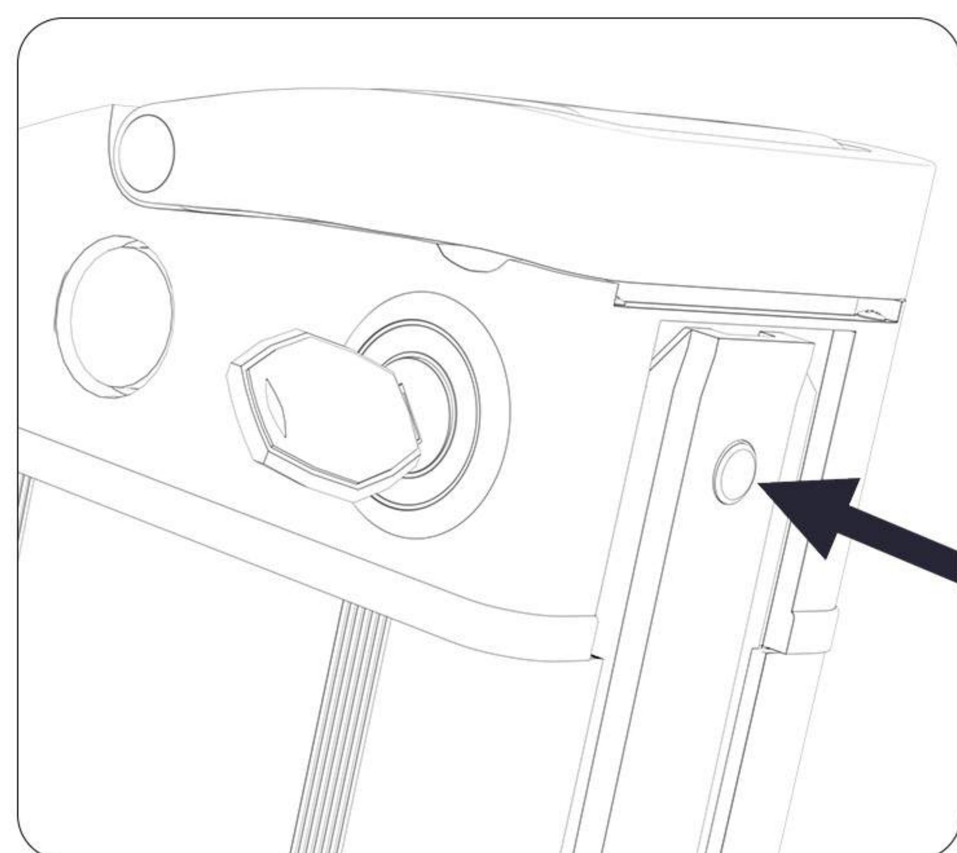
Position 2: In this position, the key can be removed, but the battery will not supply power.
