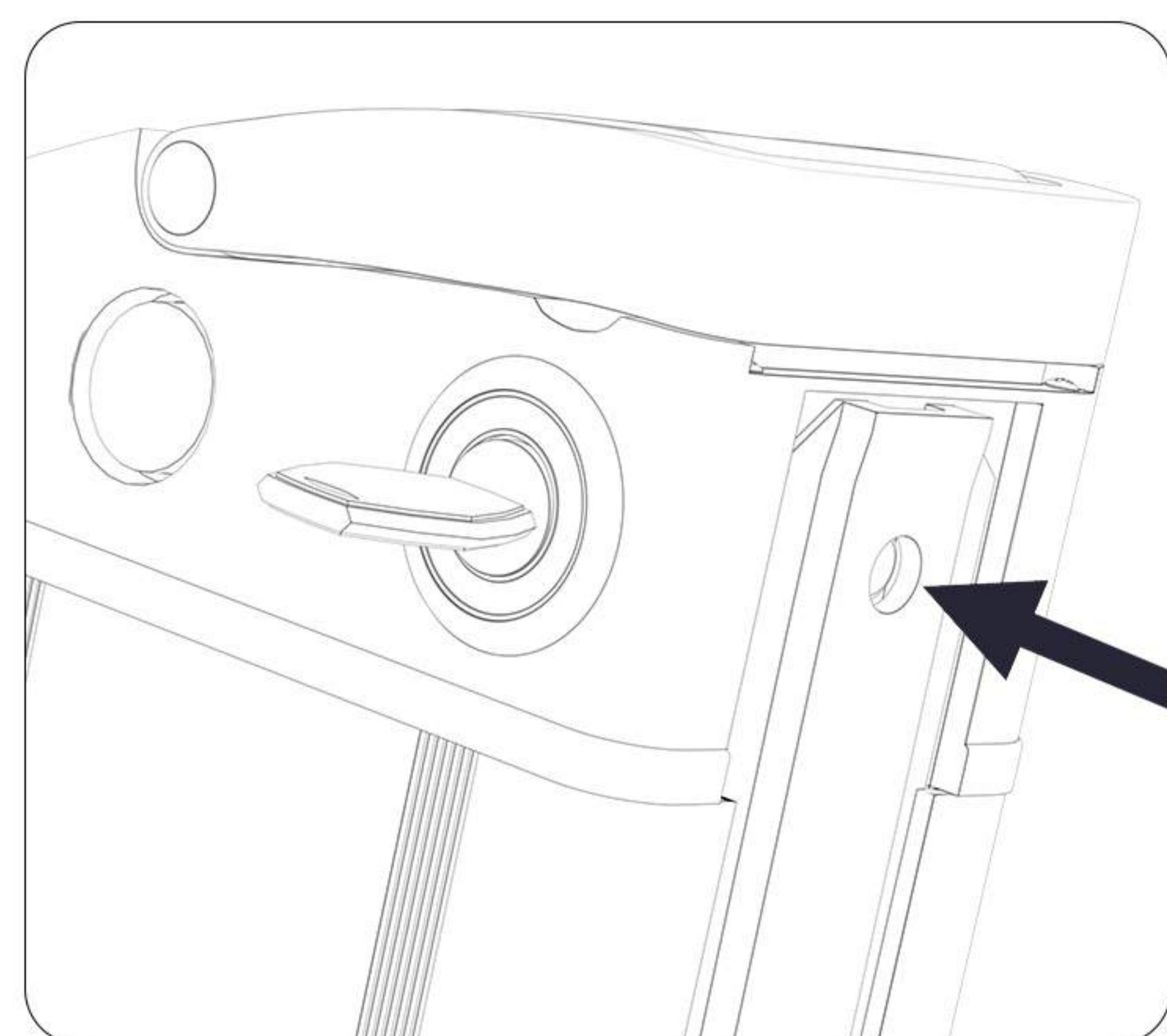
Position 3: In this position, the key can be removed, and the battery can also be taken out.
