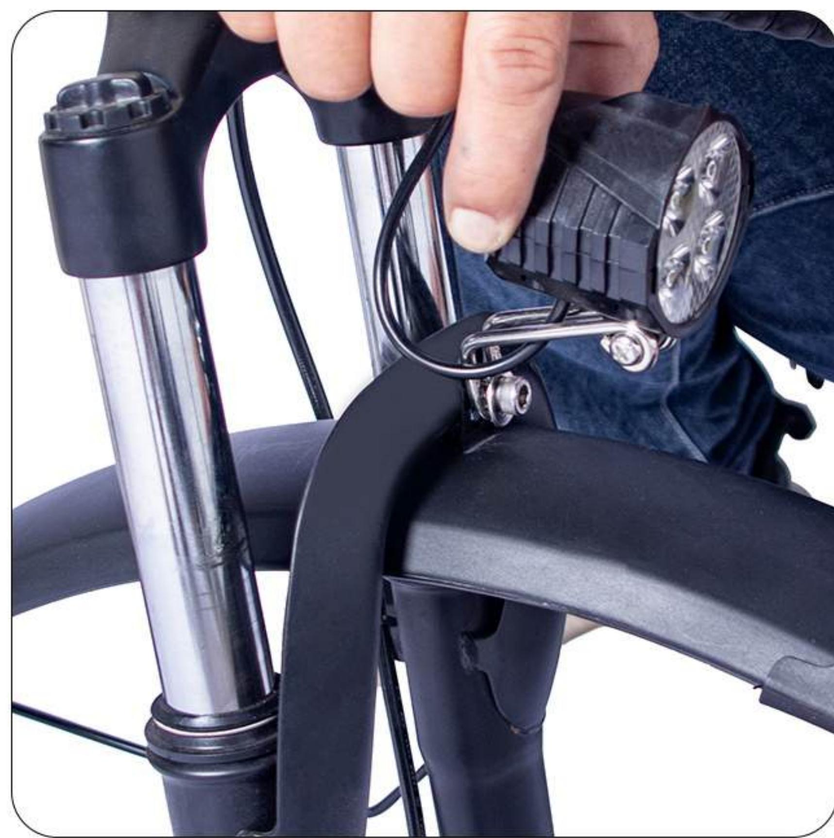
7. Install the light and fender brackets onto the front fork according to the order in the pictures.
