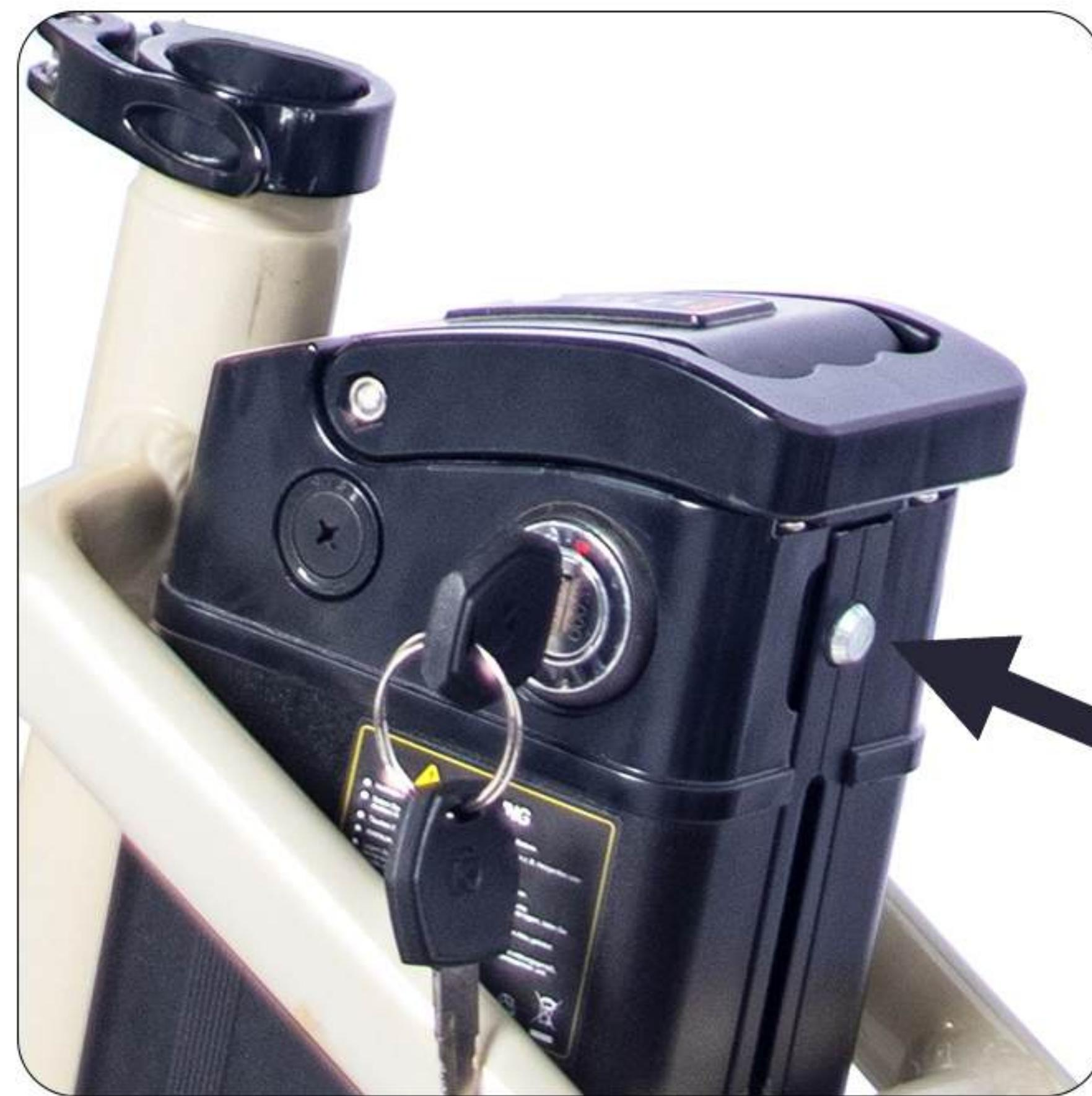
2. Turn the key to retract the rear latch into the battery.
