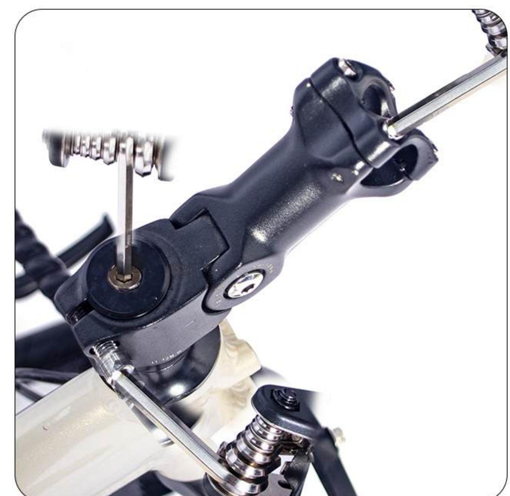
3. Adjust the Stem to the front and lock the screws with an Allen key. Use an Allen key to remove 4 bolts.
