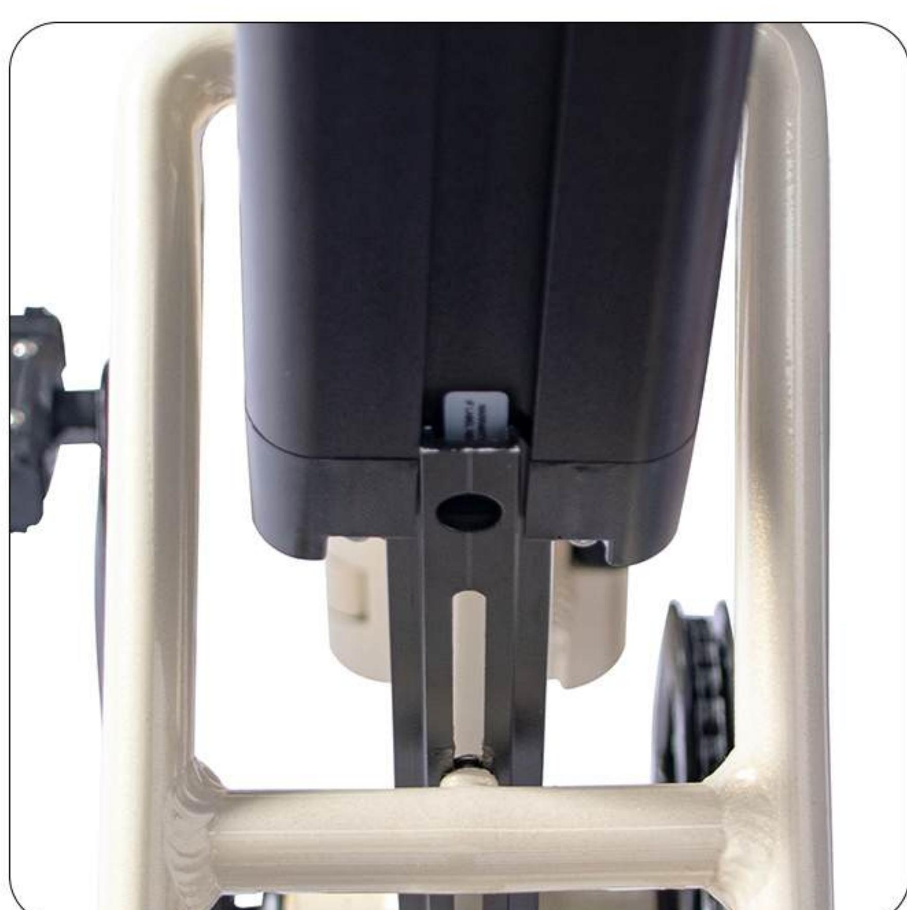
1. When installing the battery, pay attention to the battery and the rail below.
